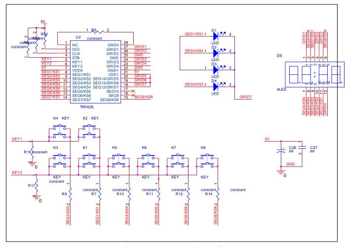
Figure 2-9 Key and Display Circuit
